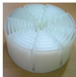
Fig.3 Metamaterial sample of electromagnetic blackhole by stereolithography
